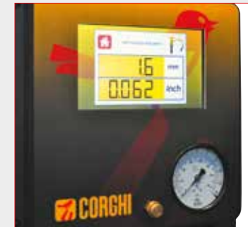
tread depth values: shown with yellow background to indicate values near minimum limit
